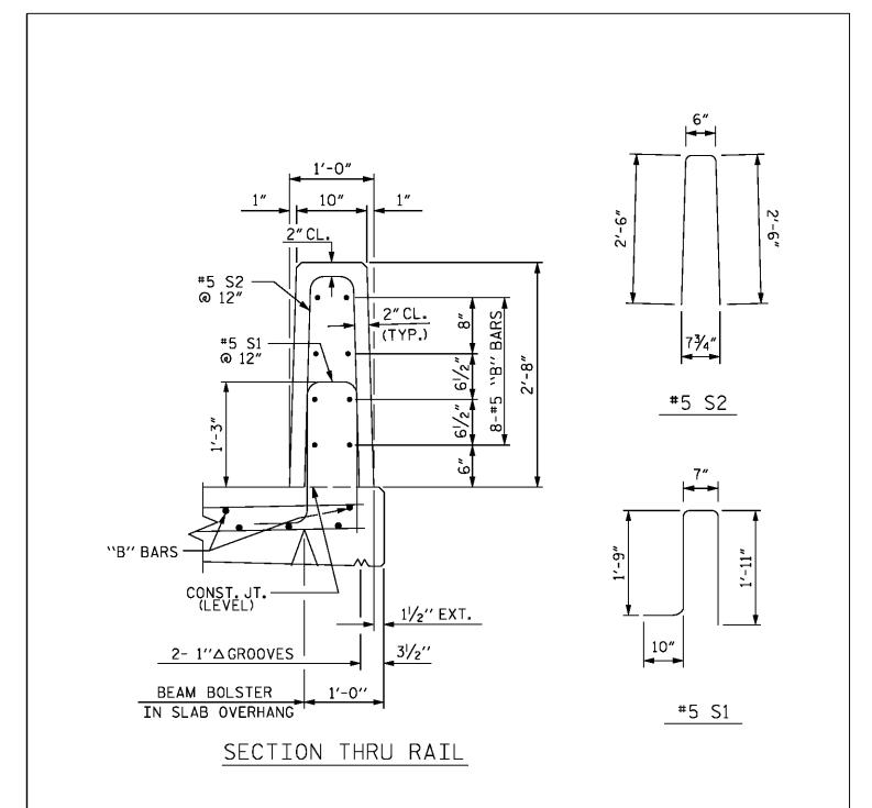
32" VERTICAL CONCRETE BARRIER RAIL
